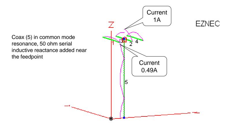
Coax in common mode resonance, 50 ohm serial inductive reactance added near the feedpoint
