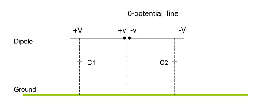
If feed to antenna is floating and C1 = C2 (symmetrical antenna), voltages settle symmetrically around 0-potential line
