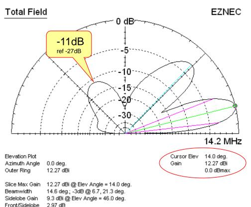
Coax in common mode resonance, 50 ohm serial inductive reactance added near the feedpoint
